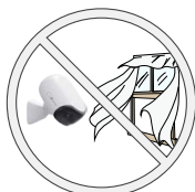
Avoid air vents or drafts (e.g., near windows)
